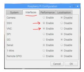
In my case, the RPi has a monitor, keyboard, and mouse only during initial setup. After that it is run "headless" (no monitor) in the "shack" and accessed from a PC running the VNC client software from <a href="http://www.realvnc.com">http://www.realvnc.com</a>
