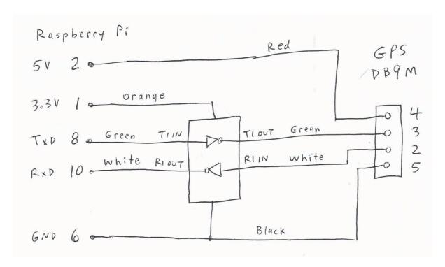
5 volts, to power the GPS, is supplied through pin 4. This is the same convention commonly used by other trackers such as OpenTrack and Tiny Trak4 so the same GPS receiver should be interchangeable between them.
