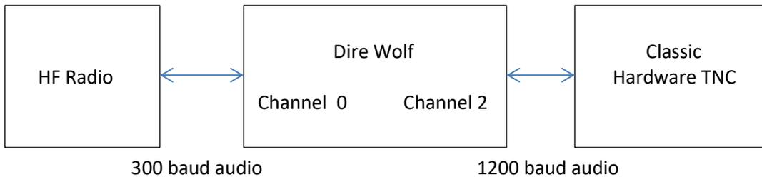
A 300 baud frame is received over the HF radio. Exactly the same thing is sent out channel 2 except at a different data rate. The TNC processes the frame and possibly sends a response. The 1200 baud packet goes into channel 2. Dire Wolf sends the same thing out to the radio, via channel 0, with a different data rate.
