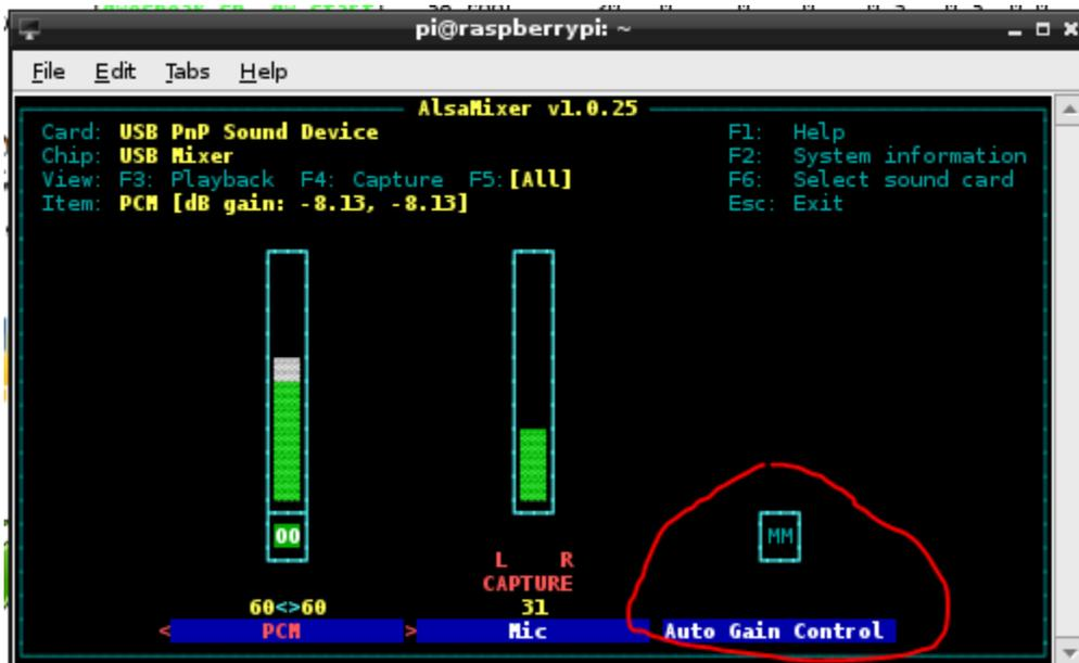
Be sure the Auto Gain Control shows "MM" which means disabled. If it shows "00," select it with the right/left arrow keys and press the "M" key so it displays "MM."
