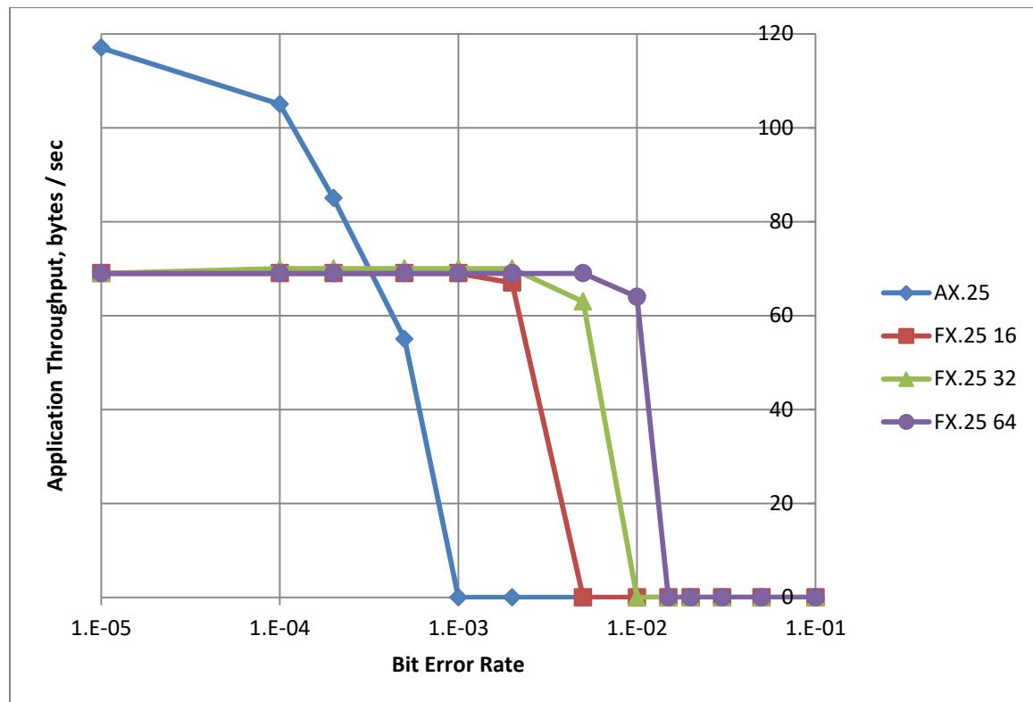
Under good conditions, FX.25 is slower because it has more overhead. When conditions deteriorate, FX.25 show little or no degradation long after AX.25 is completely useless.
