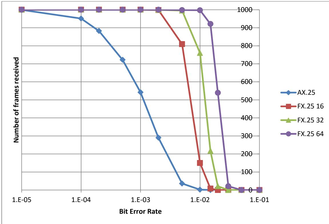
Regular AX.25 fails when even a single bit is corrupted.
