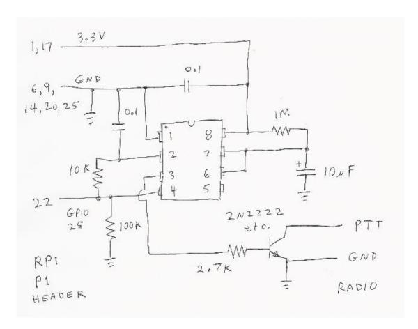
You could get by with only a resistor and transistor but a software failure could cause the transmitter to be stuck on, jamming the radio channel, annoying other people, and possibly damaging the transmitter from overheating.
