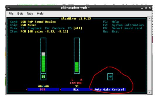
Be sure the Auto Gain Control shows "MM" which means disabled. If it shows "00," select it with the right/left arrow keys and press the "M" key so it displays "MM."
