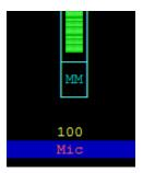
This means the input is muted. Press the "M" key to unmute. You might not be able to get the audio level input low enough if Auto Gain Control is enabled on the soundcard input. If you see something like this:
