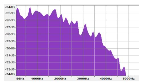
Note the peak at 4800 Hz. This corresponds to the maximum frequency of alternating 0 and 1 bits. The upper end of the audio passband needs to extend to at least 5000 Hz.
