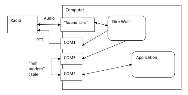
The packet radio application expects to find a TNC on COM4. COM3, connected to Dire Wolf, behaves like a KISS TNC. The two serial ports are connected to each other with a "null modem" cable. Anything coming out of the COM3 port goes into COM4 and vice versa.
