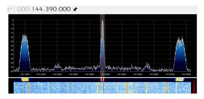
The side lobes seem to be an artifact from the SDR receiver, not a dirty transmitter. The same thing is seen with a much different transmitter.
