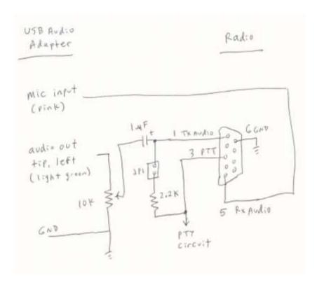
Some older hand held radios use a single pin for microphone audio and PTT. In this case, the jumper is installed so the Mic input is pulled to ground with a 2.2k resistor.
