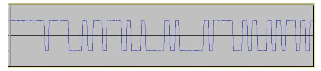
On the receiving end, we use a digital phase locked loop (DPLL), synchronized to the zero crossings, to determine where to sample for the data bits.
