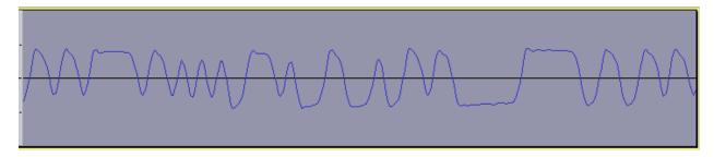
The amplitude is not that important because we slice at the zero level to get a binary value. The jitter of the zero crossing points is very important because this is where we get our timing. If the sample rate is too low, we will get more jitter.
