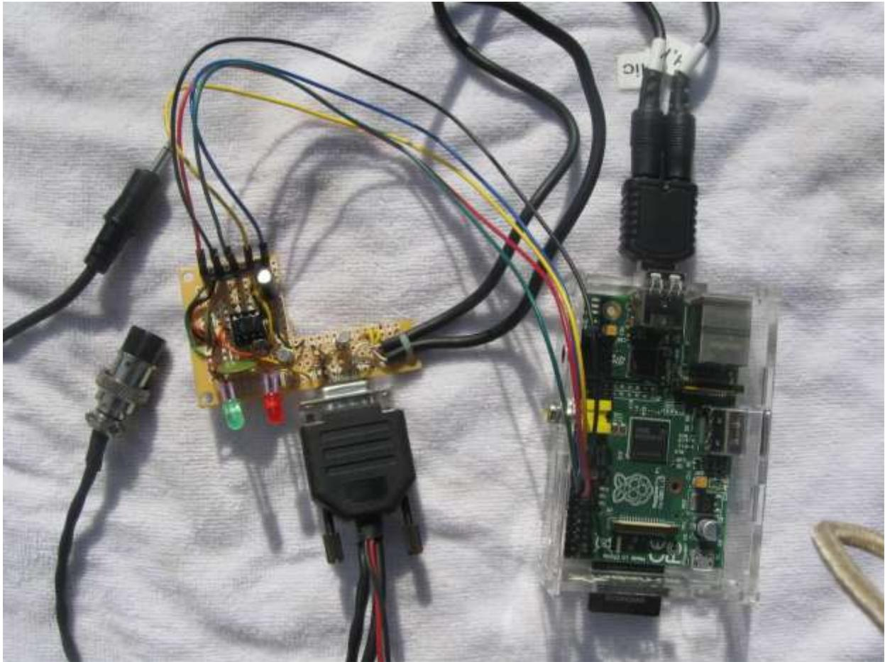
**Left:** Connections to speaker and Microphone jack of transceiver.
