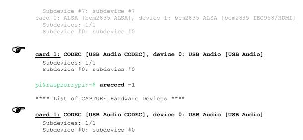
The built-in (output only) interface will normally be card 0 unless you did something to change the order. The additional USB audio adapter will typically be card 1, as seen in the example above. If you see a different number, you will have to modify a later step when we put the card number in the configuration file.
