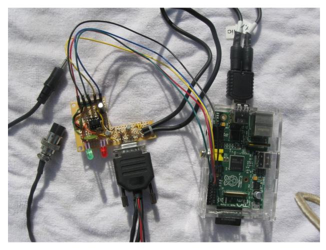
**Left:** Connections to speaker and Microphone jack of transceiver.
